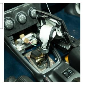
Remove the single bolt and nut connecting the shift arm to the shifter.
