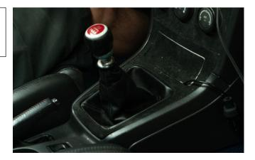
The center console trim components have clips going around their perimeters. Working your way around the trim, pull straight up and the clips will release from the center console assembly.
