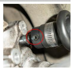
Install the new shift arm onto the shifter by using the same hardware that was used here.
