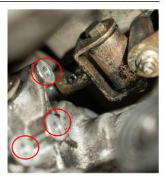
Place the punch directly over the roll pin and drive it out completely by tapping a hammer on the punch. If the roll pin is having a hard time coming loose, try soaking it in penetrating oil. This can help break it free easier.
