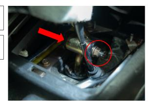
This completes the install for the Subaru Precision Shift Arm. Before driving the vehicle, it is a good idea to double check that all of the steps have been completed and all bolts are properly secured back into place. Check that the shifter goes into all gears before driving the vehicle.
