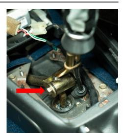
Remove the bolt securing the front of the shifter stay to the transmission
