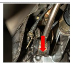
Remove the (3) bolts holding the shifter stay bracket to the transmission, this will provide additional room to access the roll pin connecting the shift arm to the transmission.
