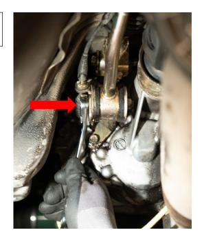
When the bolt has been removed, drop the shifter stay out from its bracket.
