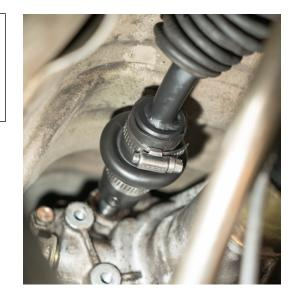
This is an example of what the roll pin should look like when it has been installed into the new shift arm and transmission shaft.
