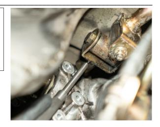
Once the roll pin has been removed, set it to the side as it will be re-installed back onto the vehicle.
